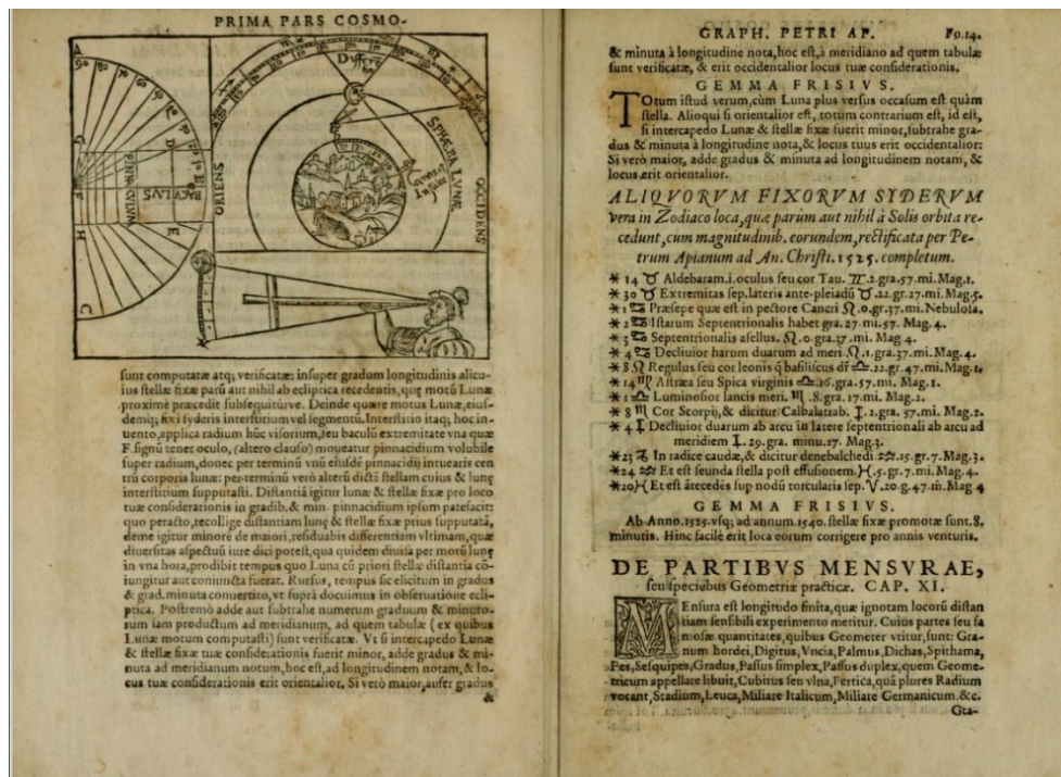
Fig. 2. Using a cross-staff to measure an astronomical angle. Apian 1564, 34. Source: archive.org .
